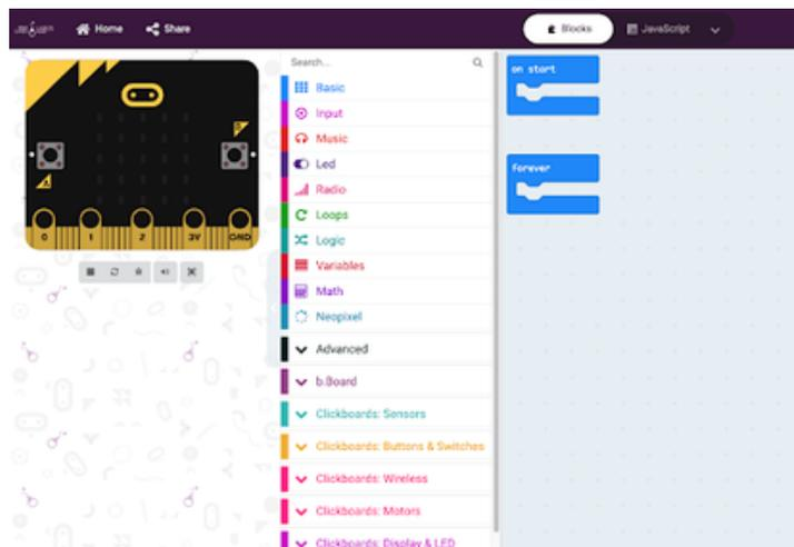
On the left hand side of the screen you can see the toolbox. This is where we keep all of the blocks of code you need to control your micro:bit and b.Board. Let's experiment with reading the soil moisture by displaying the analog value on the micro:bit LED screen. To do that, grab the 'show number' block in the basic toolbox as shown here:
