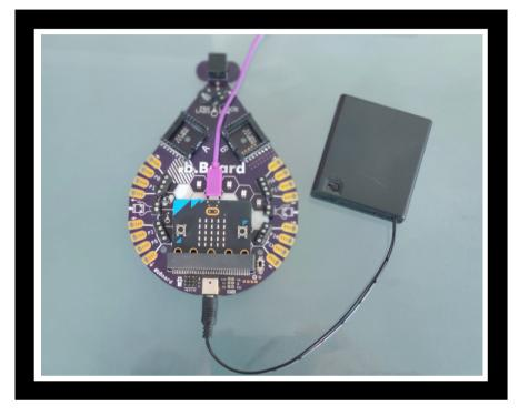
Connect the battery pack and if your pack has an on/off switch please ensure to turn on the battery pack. (Please note there are various wall chargers and battery pack that function with the b.Board so yours may look different than the picture above.
