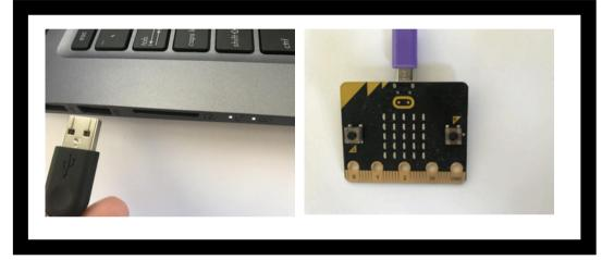
Connect the USB wire to the computer (not an iPad) and the other end of the wire into the micro:bit. If you want to use a tablet you can download the micro:bit app and flash the code.brilliantlabs.ca file via bluetooth.
