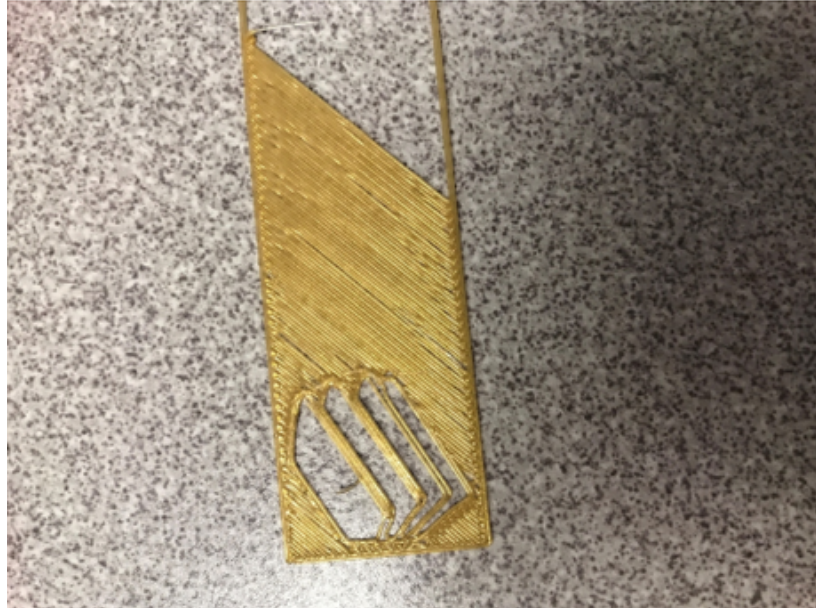
Above: A bad first layer caused by a Z offset issue. The distance between plate and nozzle is too high. Source: mrbnatural10 on 3D Hubs
