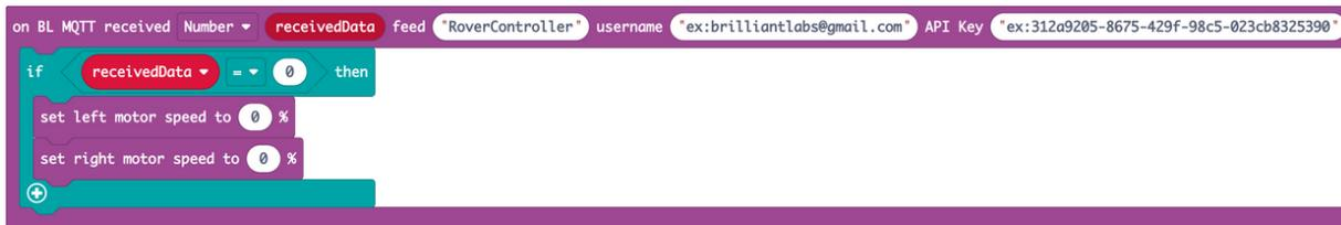
To finish up our controller, duplicate your “if” block and cover each condition for a value that the RoverController feed can send. In the example below, we’ve provided code for having the motors go forward, backward, left, right and stopping according to the values that our widgets sent when the buttons were pressed. Feel free to use this same code to drive your rover, or do something completely different, it’s up to you!
