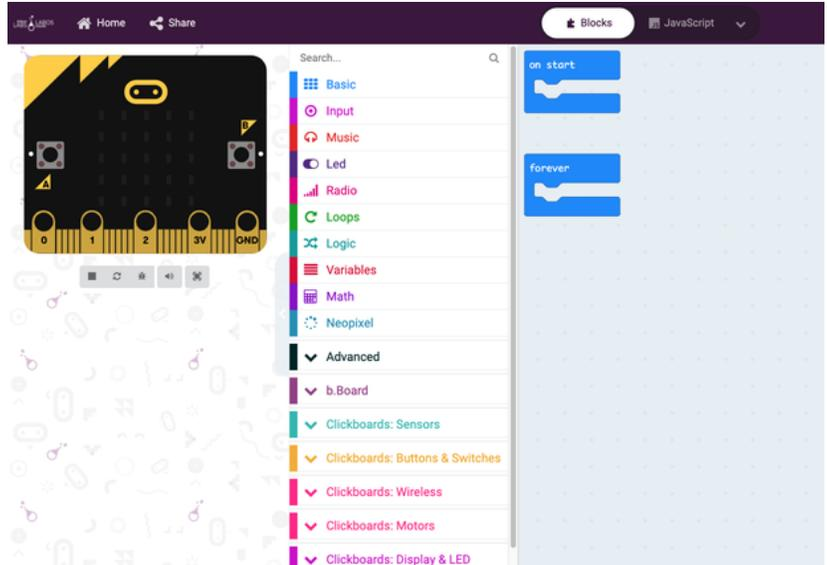
If you’re using a Click Board™ you’ll see there is a section of dropdown toolboxes where you can find the exact Click board™ you’re using. In this case, we are using the Weather click which “senses” weather, so you can find it under the ClickBoards: Sensors toolbox category here:
